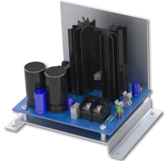
VC2000 with backplate and cartridge fuse
