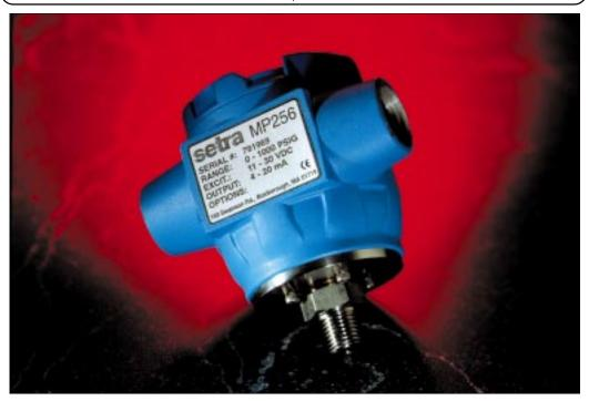
etra's Model 256 industrial pressure transducer is one of the most rugged and reliable sensors available. The Model 256 is packaged in a die-cast aluminum enclosure that is specifically designed for NEMA4/IP65 service. Setra's robust capacitive design is resistant to environmental effects, such as shock, vibration, temperature and EMI/RFI. Setra's all stainless steel sensing element does not require isolation from corrosive media.
