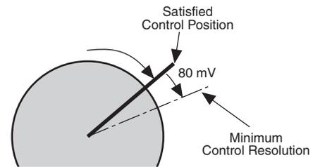
**TF Actuator responds to a 200 mV signal when reversing direction from stop position.**
