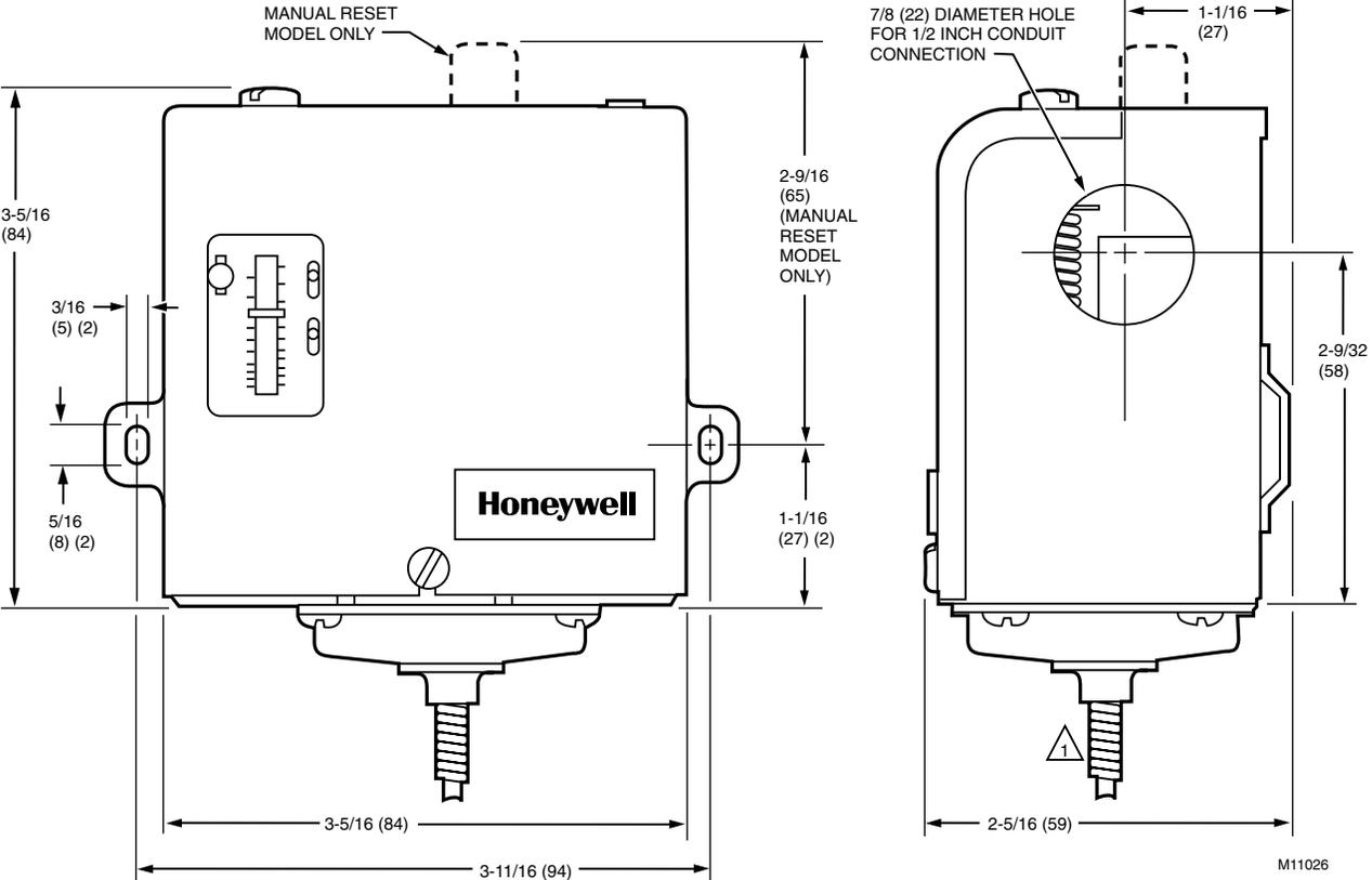
Fig. 1. L480 Temperature Controller dimensions in in. (mm).
