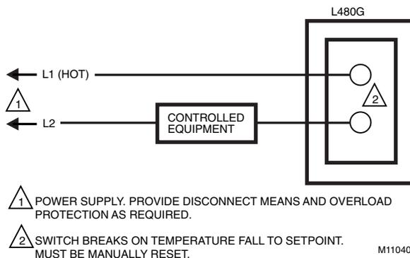
**Fig. 4. Typical hookup for L480G Temperature Controller.**
